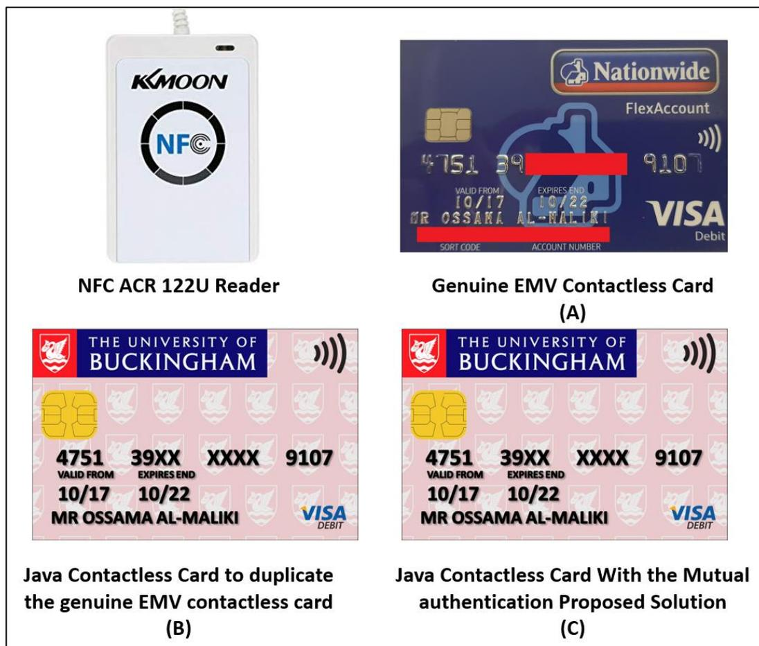
*Figure 6-3: Hardware used in the Implementations & Simulations*
